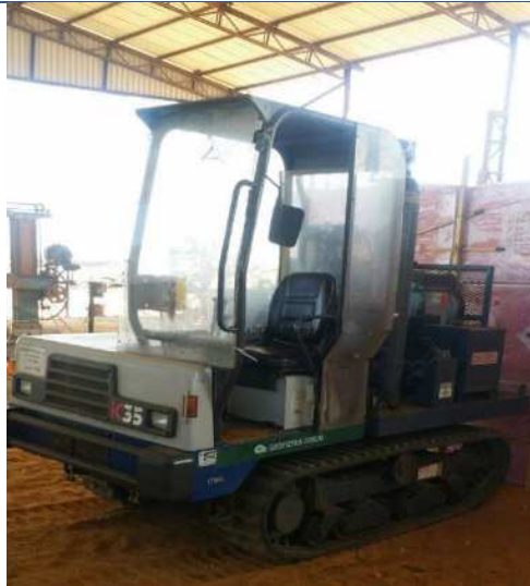
Photo 1. Light AWD vehicle used in Nhangonzo along 2 m hand cut seismic lines
